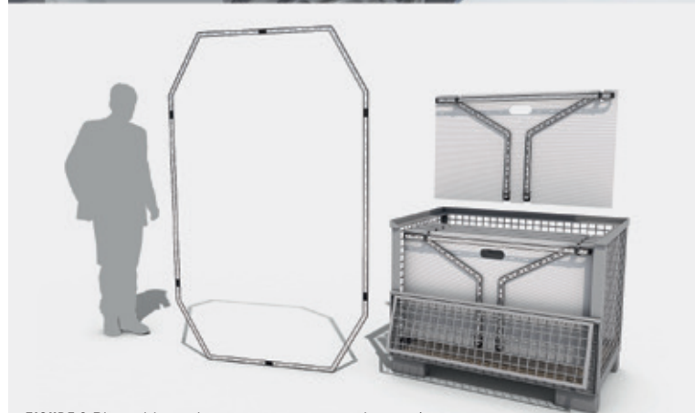
FIGURE 2 Pluggable seal test arrangement under tension, installation aid and logistics concept (© Dana)
