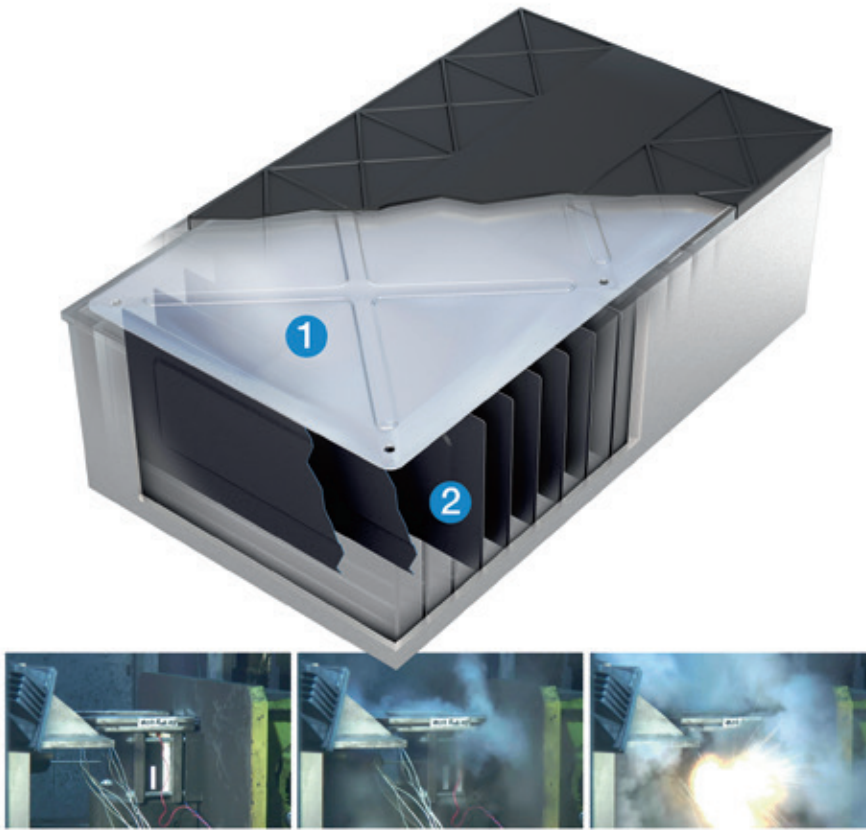
FIGURE 3 Cell module with battery heat shield (1) and swelling compensation sheet (2) – explosion caused by short-circuiting a charged cell (© Dana)
